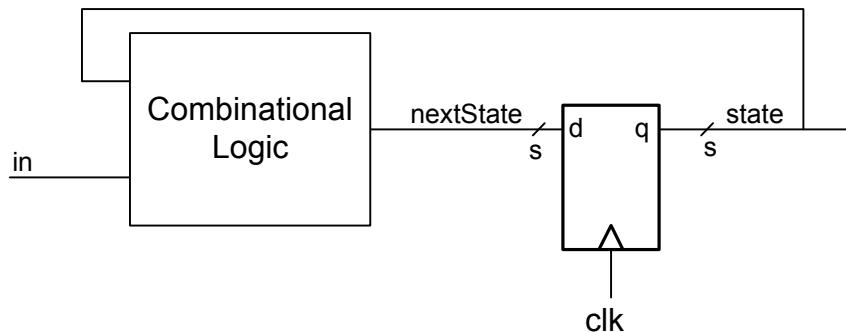
Using D flip-flops, we can build sequential logic circuits that have the form shown in the figure above. The combinational logic computes the *next state* of the circuit, an s-bit vector as denoted by the slash, as a function of the present *state* and the input. We can write this as  $\text{nextState} = f(\text{in}, \text{state})$  for some function f.
