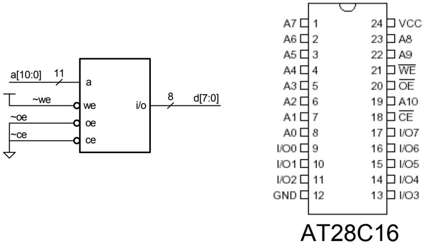
The 28C16 is a 16Kbit ROM organized as 2K 8-bit words, so the address is 11 bits wide and the constant data is 8 bits wide. A schematic symbol for the 28C16 and its pinout are shown above. Because we want the outputs always enabled we tie the low true chip enable ( $\sim$ CE) and the low true output enable ( $\sim$ OE) low. Because we are using the chip in read only mode we set the low true write enable ( $\sim$ WE) high. The write enable pin is used when programming the ROM.
