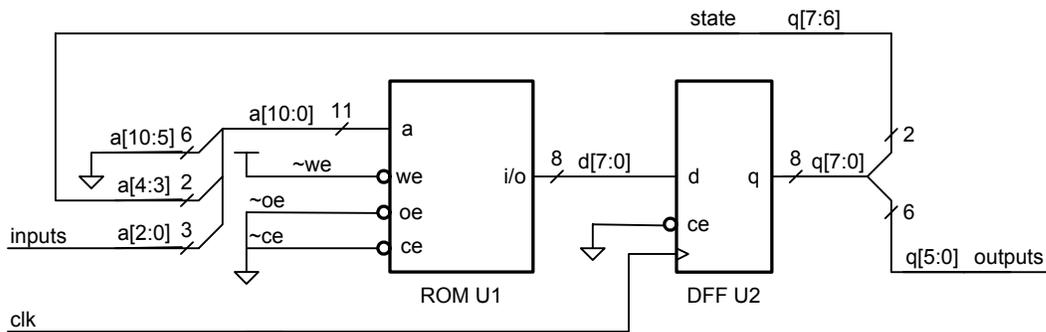
We can build a simple microcoded controller using just the ROM and an octal flip-flop (like a 74AC377) as shown above. Each cycle, the ROM calculates eight output bits  $d[7:0]$  as a function of the present state  $a[4:3]$  and the inputs  $a[2:0]$ . These eight data bits are sampled on the rising edge of the clock by the octal D-FF. The output of this flip-flop is then the current state and the outputs. This is a very simple two-chip state machine.
