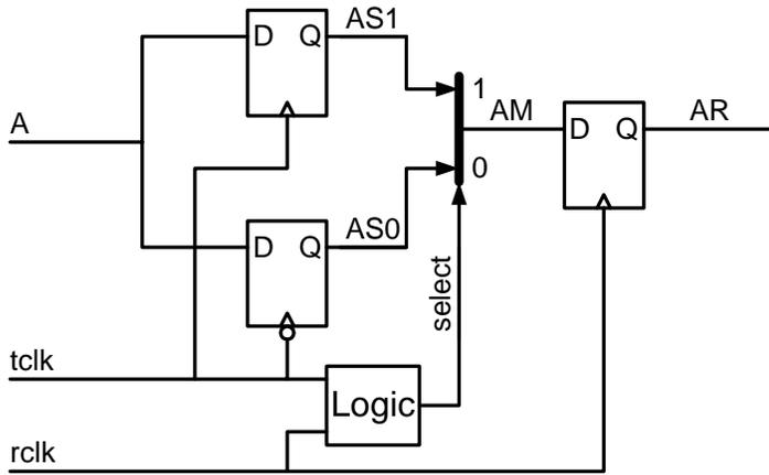
A detail of the logic block that generates select is shown below. This block samples a delayed version of tclk with rclk to decide which input of the multiplexer to select.
