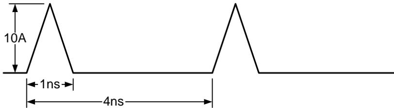
Part A [7 points]: The on-chip portion of the distribution network is modeled by the circuit shown below with 10 milli-Ohm series resistance on power and ground feeding a current source with the profile shown above. Given this load and resistive network, what is the minimum value for the local bypass capacitor,  $C_1$ , that will keep the total drop (the difference between  $V_A$  and  $V_L$ ) on the supply voltage across the load less than 0.1V?
