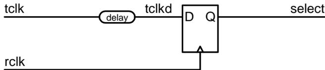
Part A [6 points]: There is something fundamentally wrong with the logic block above. What is it? Sketch a corrected logic block below. (Note, for parts A and B, assume that the signal select can switch on any symbol. It does not have to wait for a NULL on the line. We will revisit this in part C.)
