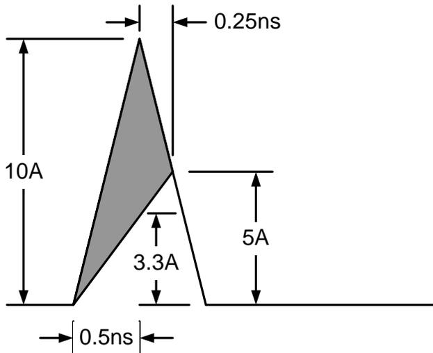
The charge is thus  $Q = 0.5(6.7A)(0.75ns) = 2.5nC$  (Alternatively you can just note that this is half the area under the curve.) To keep the voltage drop to 0.1V, the Capacitor must be sized  $C_1 = Q/\Delta V = 2.5nC/0.1V = 25nF$ .
