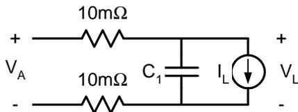
With a maximum drop of  $\Delta V = 0.1$ , the resistors supply a current of  $\Delta V/R = 5A$ . If we approximate the ramp in resistor current as linear, then the charge that must be supplied by the capacitor is the area of the shaded region in the figure below
