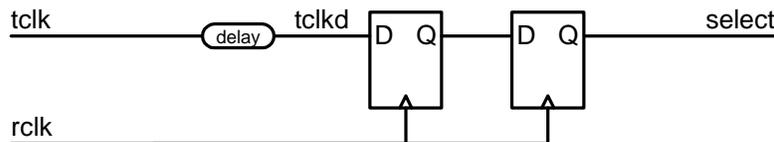
Part B [6 points]: What is the proper value for the delay element in the logic block above (as a fraction of a clock cycle)? Give the value that maximizes timing margins. To keep things simple, assume that clock-to-Q delay is zero and that  $t_s = t_h$ .
