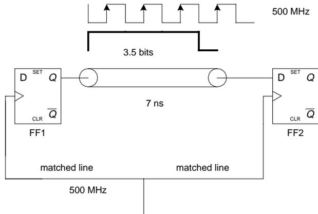
Let the data on the link travel from FF1 to FF2. The delay of the link,  $T_{\text{wire}} = 7 \text{ ns}$ .
