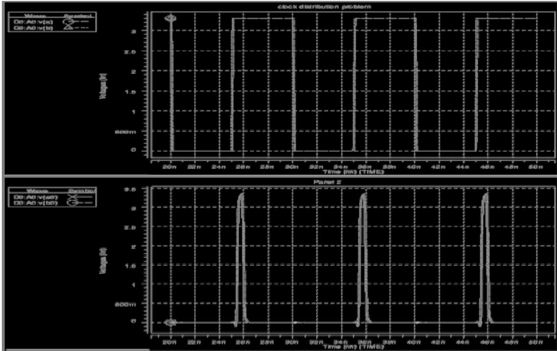
Luckily, we're on the safe side. Note that  $a_0$  and  $b_0$  goes high when the phase offset is very small.  $b_0$  going high is not predicted by the no-delay interpretation of the table.
