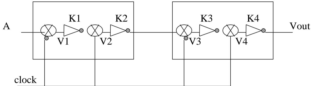
In this scenario, no flip-flops contain any regenerative gain stages. Therefore, no matter how long the waiting time is, it is possible that the output may never switch in the right direction.
