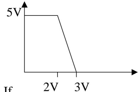
Suppose now that the input  $A$  comes in, uniformly distributed such that  $P_a = t_a \cdot f_{clock}$ .  $\Delta V_1$  will form at the output of inverter 1. This voltage is then gained up by the subsequent inverters to give a final voltage at  $V_{out}$ . If this voltage  $0V < V_{out} < 5V$ , then there will be a synchronization failure.
