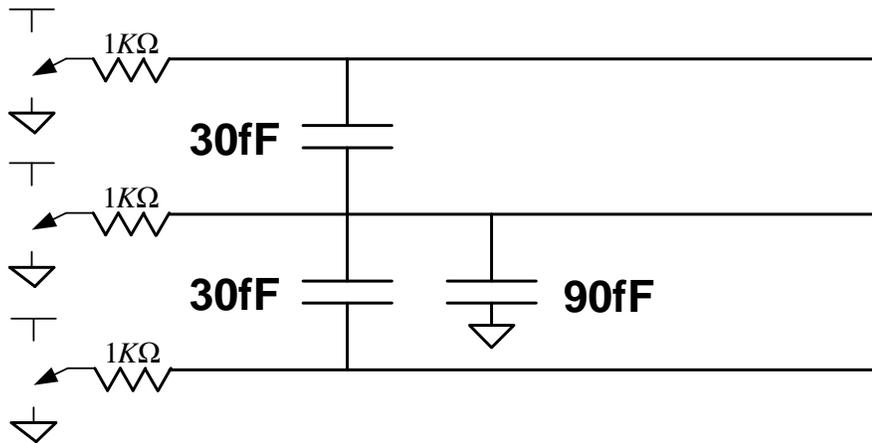
The middle line will transition fastest if the two adjacent lines are switching in the same direction, effectively eliminating the 30fF coupling capacitances. Thus, the data sequences that will result in the middle line switching the fastest are:  $\boxed{111 \rightarrow 000}$  and  $\boxed{000 \rightarrow 111}$
