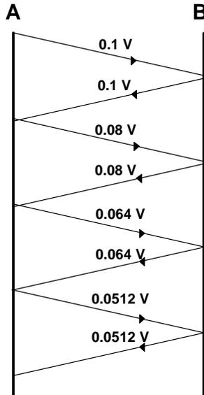
The termination is open, so we get complete reflection of the incident wave – i.e. the reflection coefficient at the termination is  $k_{rt} = 1$ . The reflection coefficient at the
