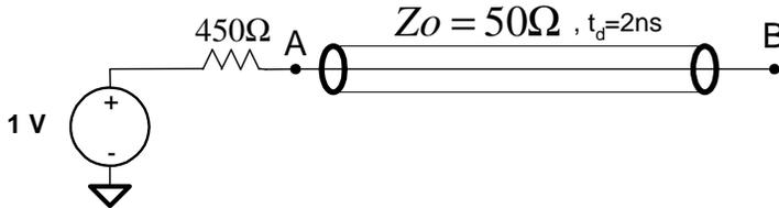
The voltage at point A immediately after the 1 V step is applied is:
