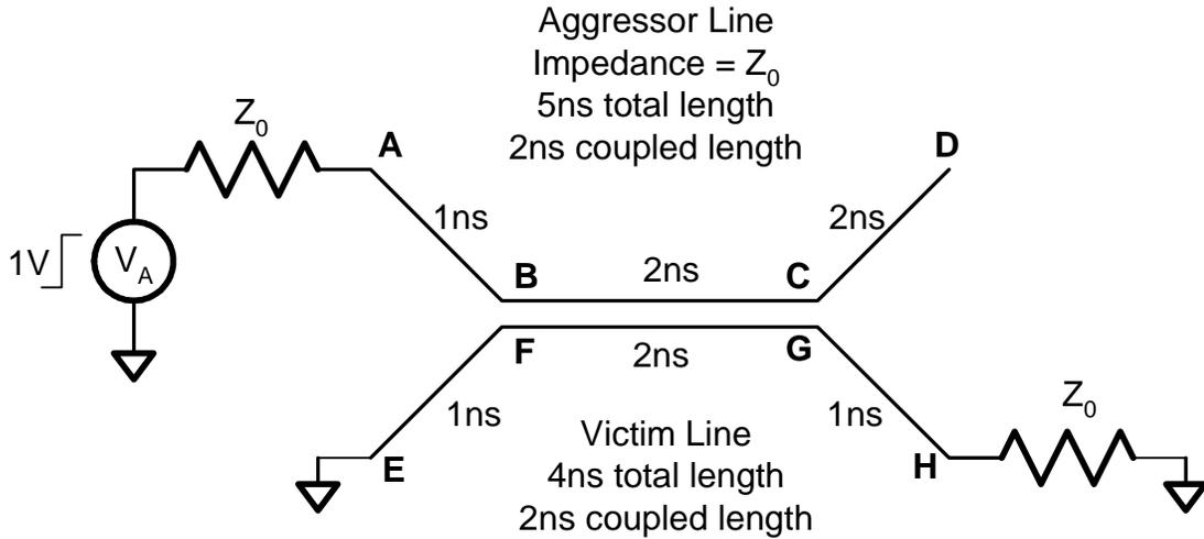
Using this information, sketch and dimension the voltage waveform at the far-end of the victim line (point H). You may ignore any effects that lead to waves with less than 10mV amplitude.
