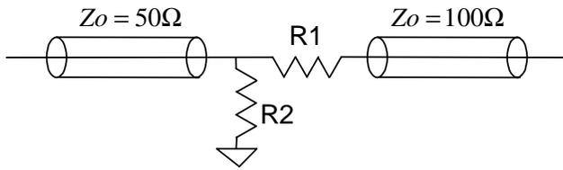
To pass a wave traveling in either direction without reflections, we solve the two equations:
