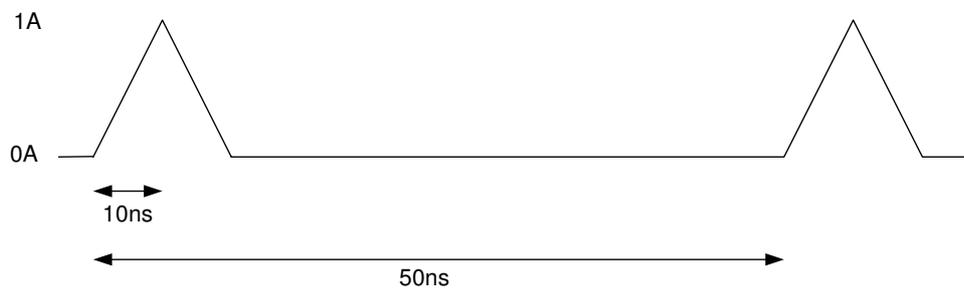
We begin by calculating the required Capacitance,  $C_B$ , for the bypass capacitor without shunt regulation. Our maximum voltage ripple is:
