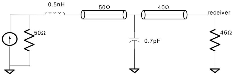
First, you can see from the TDR that there are inductance and capacitance and two transmission lines.
