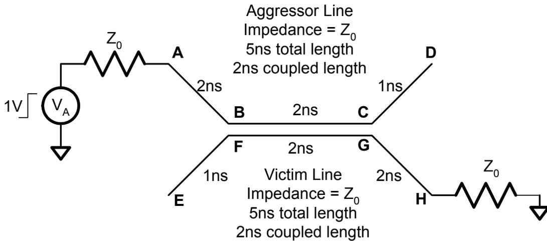
Using this information, sketch and dimension the voltage waveform at point G on the victim line. You may ignore any effects that lead to waves with less than 10mV amplitude.
