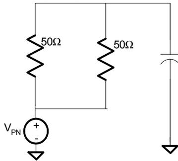
$$\text{Reference Delay} = RC = 25\Omega \cdot 100\text{pF} = 2.5 \text{ ns}$$
