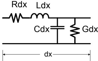
At 100 KHz,  $R \gg \omega L$ . Also the impedance presented by  $L = L/tr$  is small.
