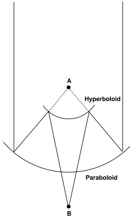
Figure 2: *The Cassegrainian telescope configuration* Point  $A$  is where the focus of the paraboloid and the virtual focus of the hyperboloid coincide. Point  $B$  is the real focus of the hyperboloid.
