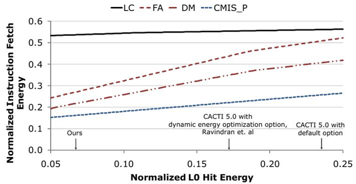
(f) Sensitivity of energy saving on the L0 to L1 access energy ratio. Normalized L0 hit energy denotes the hit energy of the 256-instruction DM normalized to that of L1.
