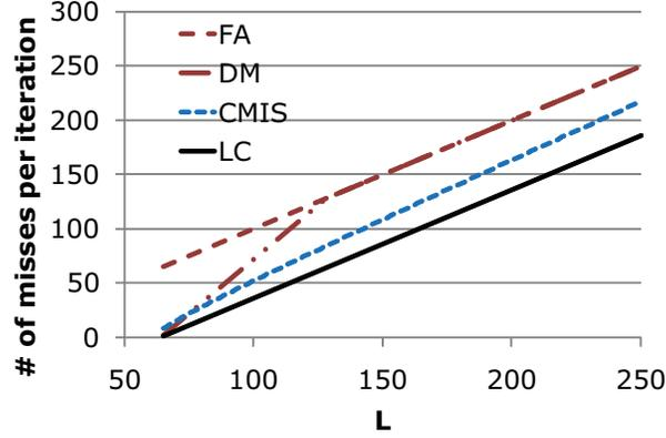
Figure 4: The number of misses per iteration for straight-line loops where  $C = 64$
