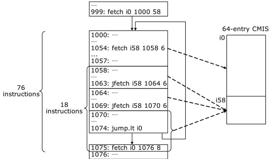
Figure 3: A code snippet of a loop and its mapping to a 64-entry CMIS
