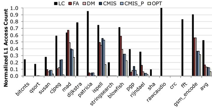
(b) The number of L1 accesses. Each shows the number of L1 accesses normalized to the baseline, in which no L1 access is filtered.
