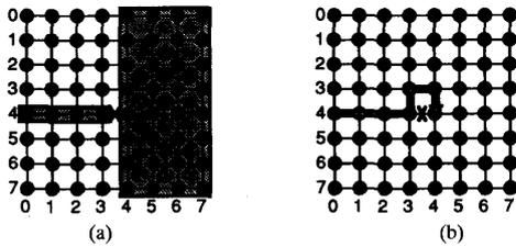
Fig. 2. An 8-ary 2-cube network with a faulty channel from  $(3, 4)$  to  $(4, 4)$ . (a) With dimension order routing, packets from the shaded area on the left to the shaded area on the right cannot be delivered. (b) Using adaptive routing packets can be delivered between all pairs of nodes.
