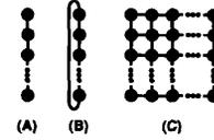
Fig. 3.  $k$ -ary  $n$ -cube is a cube of  $n$  dimensions with  $k$  nodes in each dimension. (a) Meshes are cubes with each dimension connected in a linear array. (b) Connecting each dimension in a ring gives a Tori. (c) Higher dimensional cubes are constructed by combining like elements of lower dimensional cubes.
