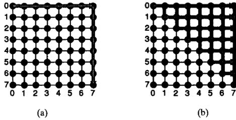
Fig. 1. Routing packets in an 8-ary 2-cube from  $(i, 0)$  to  $(7, i)$  (for  $i \in [0, 7]$ ). (a) Using dimension order routing, seven packets must traverse the channel from  $(6, 0)$  to  $(7, 0)$ . (b) Using adaptive routing, all packets proceed simultaneously increasing throughput by a factor of 7.
