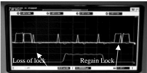
**Figure 10:** Receiver showing loss of lock and regain of synchronization with transmitter
